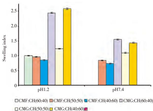
**Figure 3.** Swelling indices of the formulated CMF–CH or CMG:CH IPC films in pH 1.2 (2h) and pH 7.4 (24hrs). Data is represented as mean±SD.
