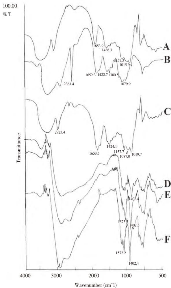
**Figure 2.** FTIR spectra of GG (A); CH (B); CMG (C); complex formed by interacting CMG and CH in the ratio of 40:60 (D); 50:50 (E) or 60:40 (F)
