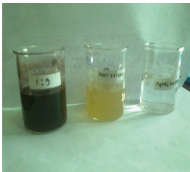
Figure 1. Synthesised nanoparticles changes color after mixing of silver nitrate and Parthenium root extract (1:9) during 48 h.
